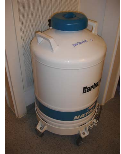
Stockage azote liquide
